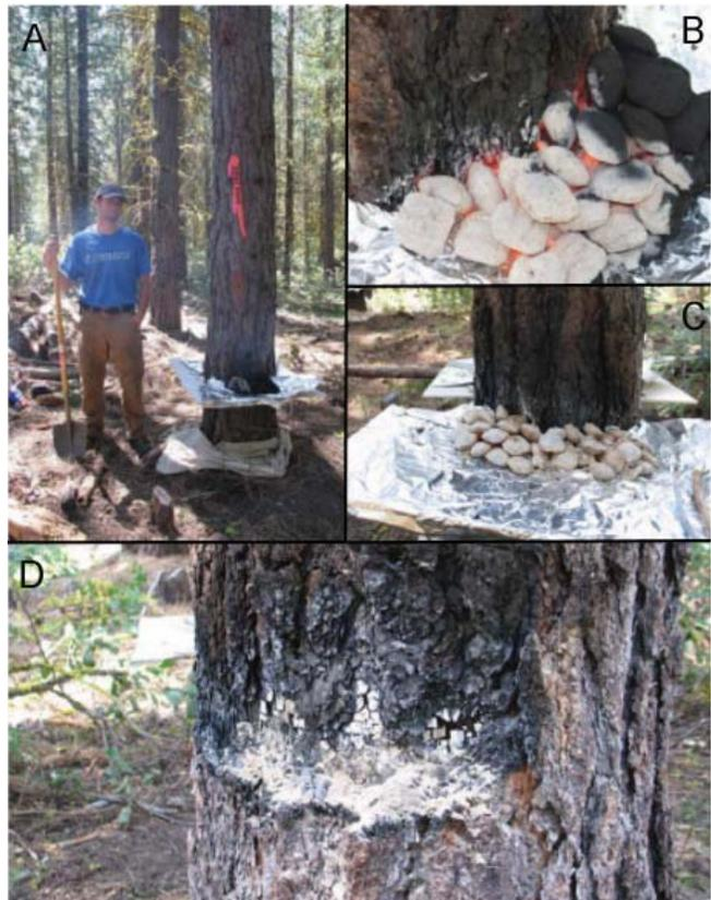
Bole charring treatment photos. Clockwise: A-Platforms and charcoal briquettes assembled and ignited; B-Close-up of burning briquettes; C-Position of briquettes around bole after combustion; D-Close-up of the burn scar on one side of a treated tree.
