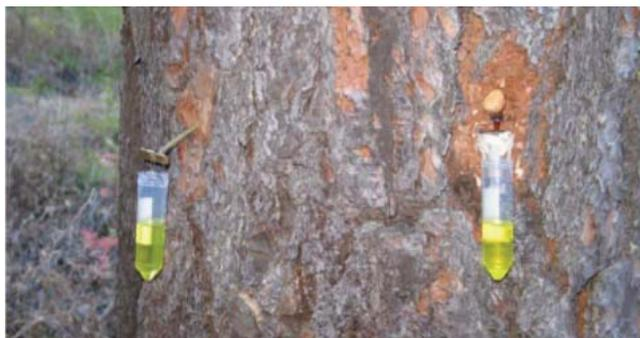
Example of measuring resin flow using two different methods on one tree at Leavenworth, WA. The scoop method is on the left, and the exposed xylem of the arch-punch scar is visible on the right. For additional details see the team’s final report.
