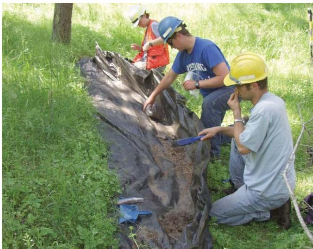
Silt fence installed lengthwise across the slope allowed scientists to collect and measure the amount of eroded materials.
