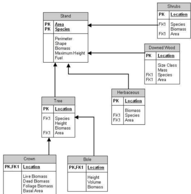
Visual description of a data model for forest fuel attributes measured from remotely sensed data. Elements can potentially be measured via remote sensing, and values can be computed using GIS (figure from JFSP final report).
