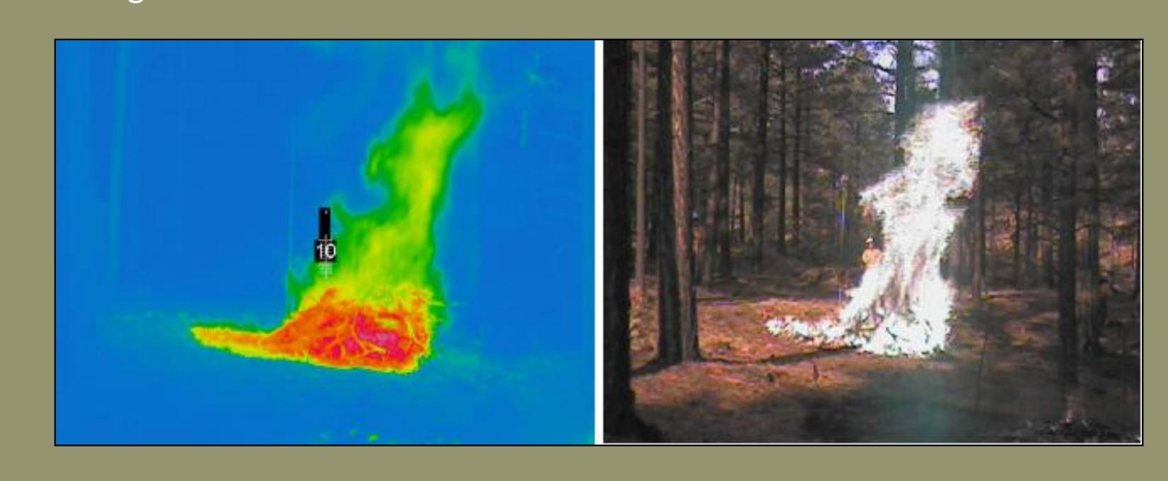
We are measuring aboveground heat flux with an infrared camera (above) and buried thermocouples (below, left) that measure below-ground temperature and duration of heating during the burn (below, right).
