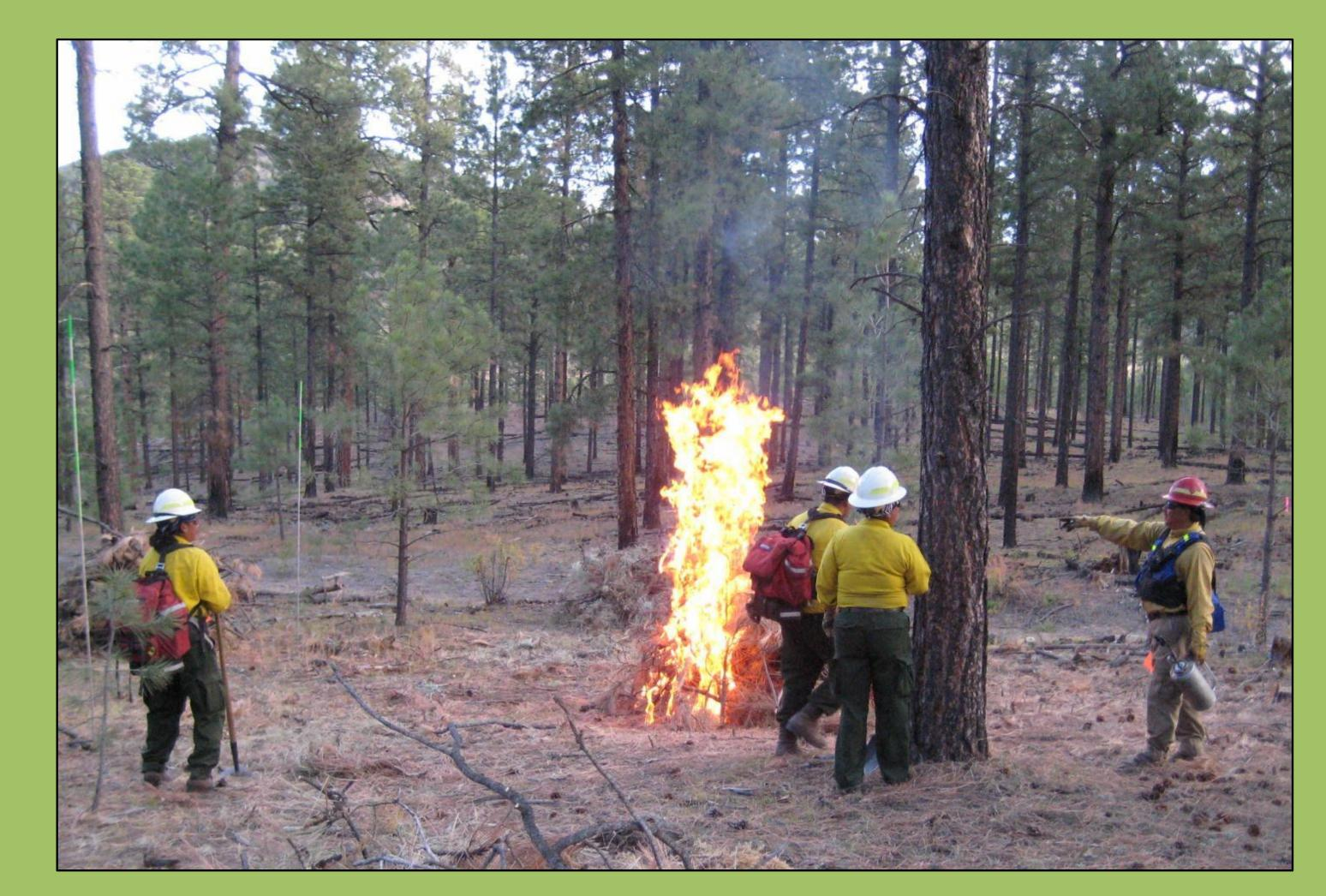
We time the burns and record flame height. In the fall of 2011 flaming combustion was over in about 30 minutes, but piles continued to smolder for more than 12 hours. Once the ash is cool, we collect unburned material and charcoal to see how much biomass is consumed, and how much charcoal is produced.
