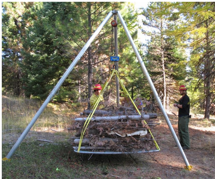
Figure 5. Pile mass loss measurement apparatus.
