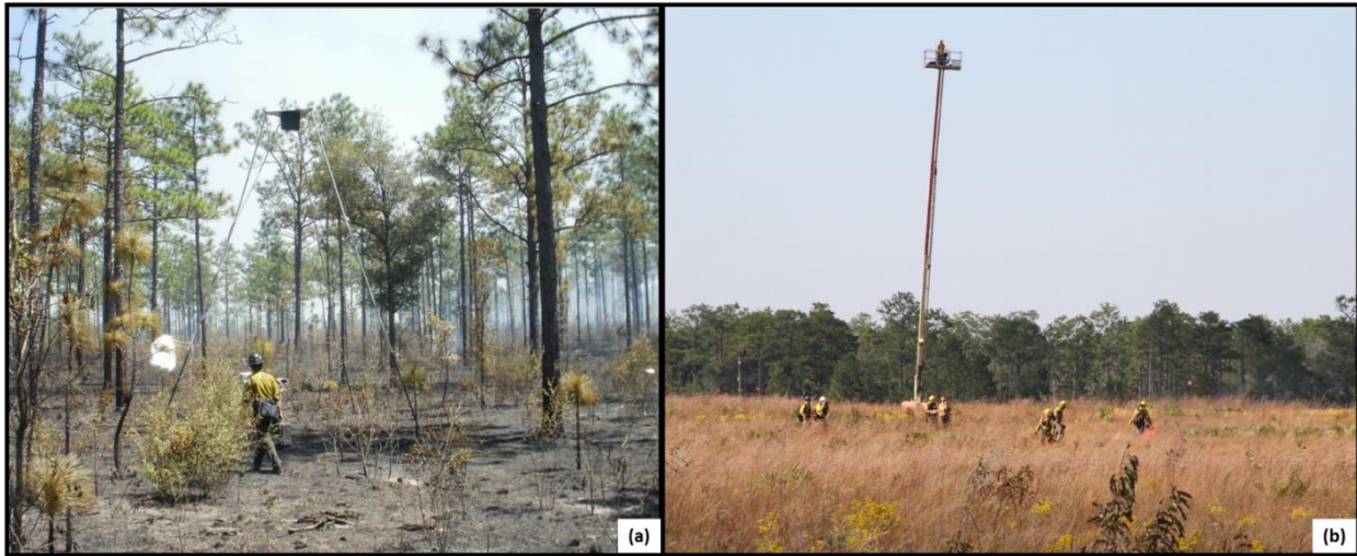
Figure 9. (a) Tripod system and (b) boom lift used to collect nadir and oblique Long-wave infrared (LWIR) thermographic measurements, respectively, of surface wildland fires.
