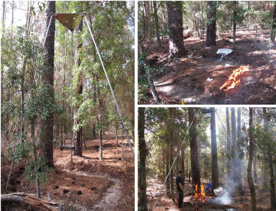
Figure 1. Panel (a) shows plot layout. Stars represent fuel measurement locations, while x's mark thermocouple locations. Panel (b) shows Temperature monitoring equipment including large tripod for thermal infrared camera and datalogger with thermocouples.
