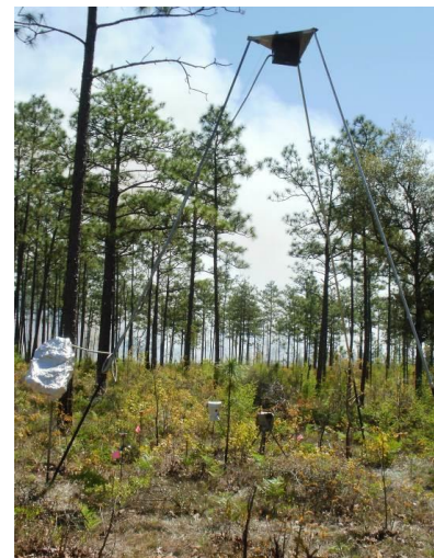
Figure 2. FLIR tripod system suspended above the HIP and deployed in advance of the fire front.
