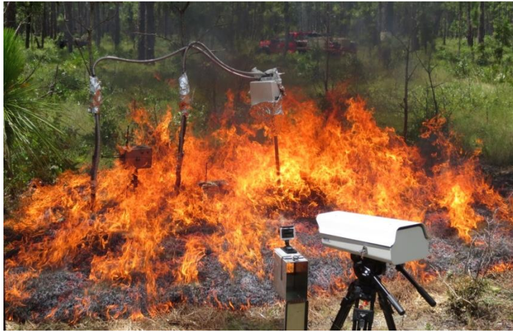
Figure 3. The experimental setup for the stem heating experiment showing FBP, FLIR, visual imagery and datalogger set up.
