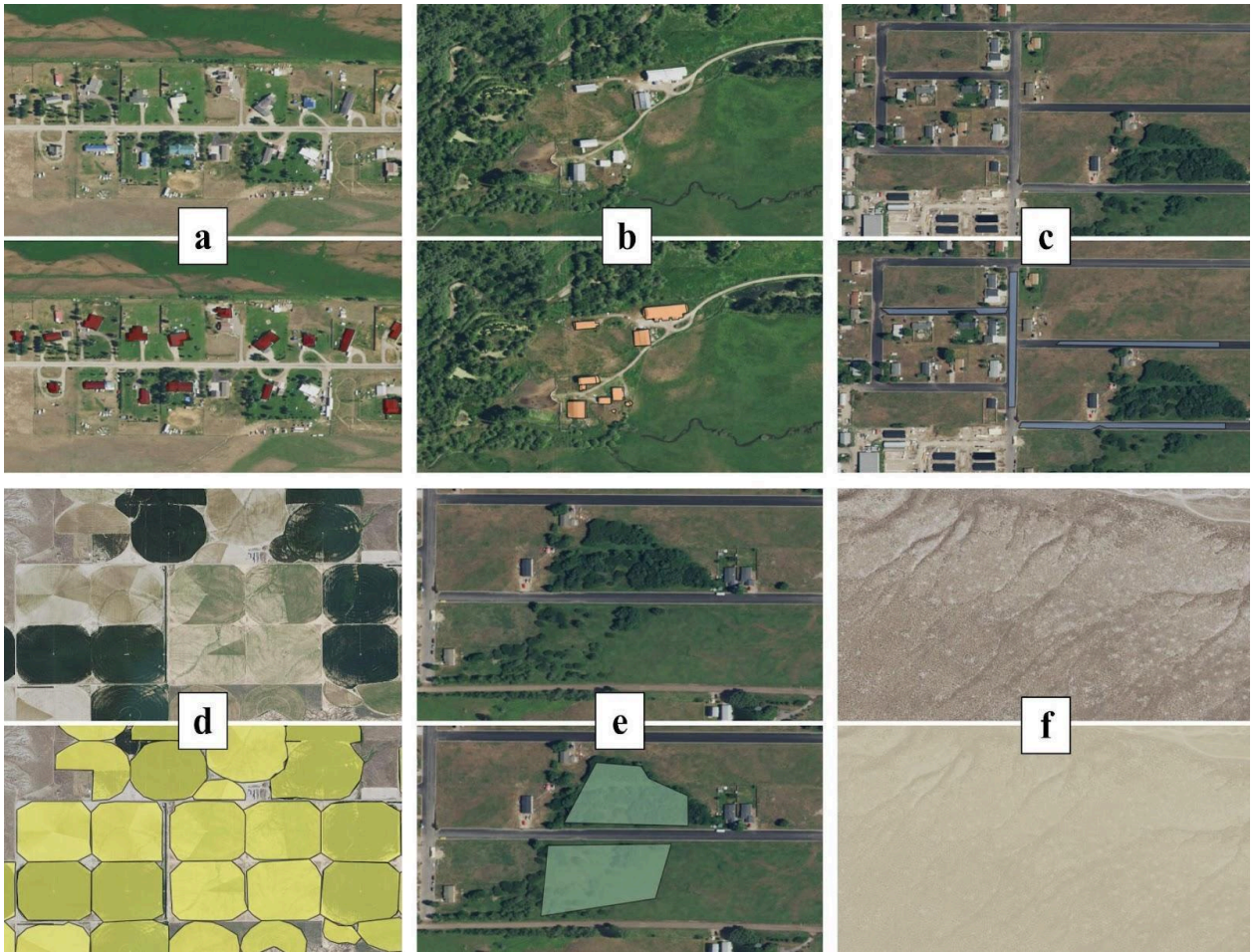
Figure 3. Comparing NAIP aerial imagery to digitized polygons for each LULC class in our workflow ((a) Residential, (b) Infrastructure, (c) paved, (d) Agriculture, (e) Vegetation, (f) Range/Scrub).
