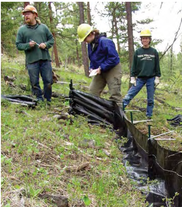
Example of a sediment fence used to measure postburn hillslope erosion.
