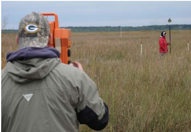
Surveying marsh plot elevations in a Schoenoplectus americanus marsh is an important step in establishing a SET-MH study site.
