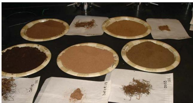
Soil samples reveal stark color differences between different burn severities. Credit: Cassie Hebel.
