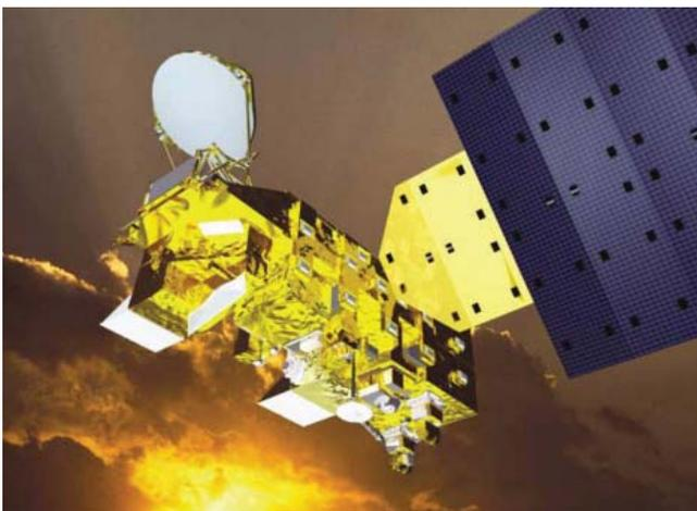
A computer rendering of the Aqua satellite spacecraft done by Reto Stöckli, based on earlier versions. This satellite is part of NASA's Earth Observing System, that delivers data on fires actively burning and areas recently burned through the onboard MODIS instruments. Credit: [http://aqua.nasa.gov/doc/pubs/Aqua\\_brochure.pdf](http://aqua.nasa.gov/doc/pubs/Aqua_brochure.pdf), Aqua brochure.
